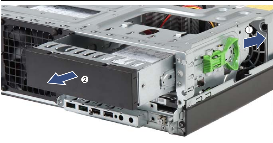
Figure 40: Removing the 5.25-inch dummy cover with HDD out of the the chassis bay
